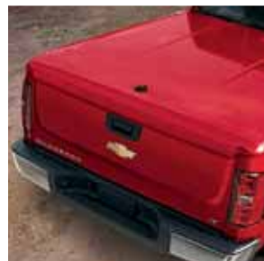
A hard tonneau cover features struts for easy opening and closing, a lock, and a quick-release mechanism.
