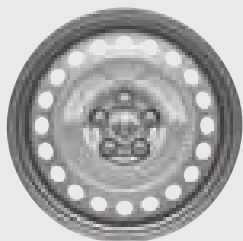
16-inch Steel Wheel with Center Cap Standard on Tradesman® Cargo Van/Wagon (WDL)
