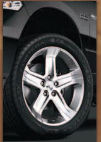
22-INCH POLISHED FORGED ALUMINUM WHEEL (STANDARD ON REGULAR CAB R/T)
