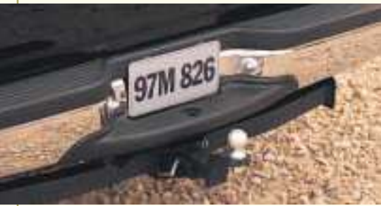
7-wire trailer wiring harness and frame-mounted hitch receiver (shown with aftermarket hitch equipment).
